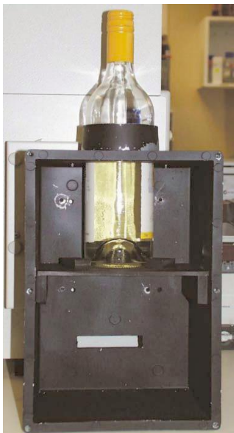
Figure 1A: Presentation of a wine bottle to a NIR spectrophotometer to measure composition.
