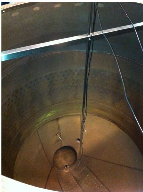
Figure 2.8: Temperature sensing equipment mounted in an empty 5-tonne fermenter
