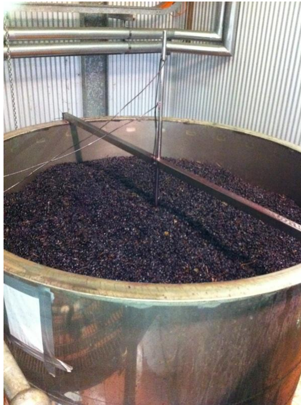
Figure 2.9: Loaded 5-tonne fermenter with temperature sensing equipment mounted
