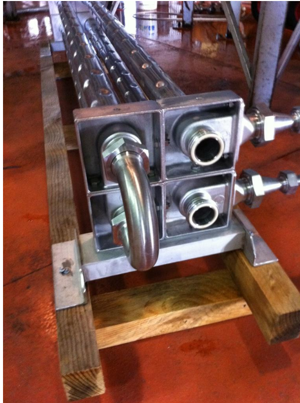
Figure 2.7: Dimpled tube-in-tube heat exchanger
