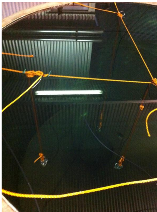
Figure 2.5: Rope and chain weights used to fix temperature sensor locations
