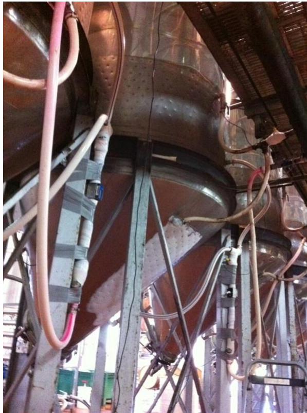
Figure 2.4: 5-tonne open-topped fermenters with brine connection lines and instrumentation shown
