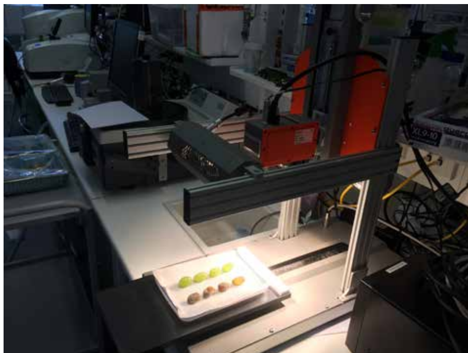
Figure 1. Specim FX10 Vis-NIR hyperspectral camera with linear stage.
