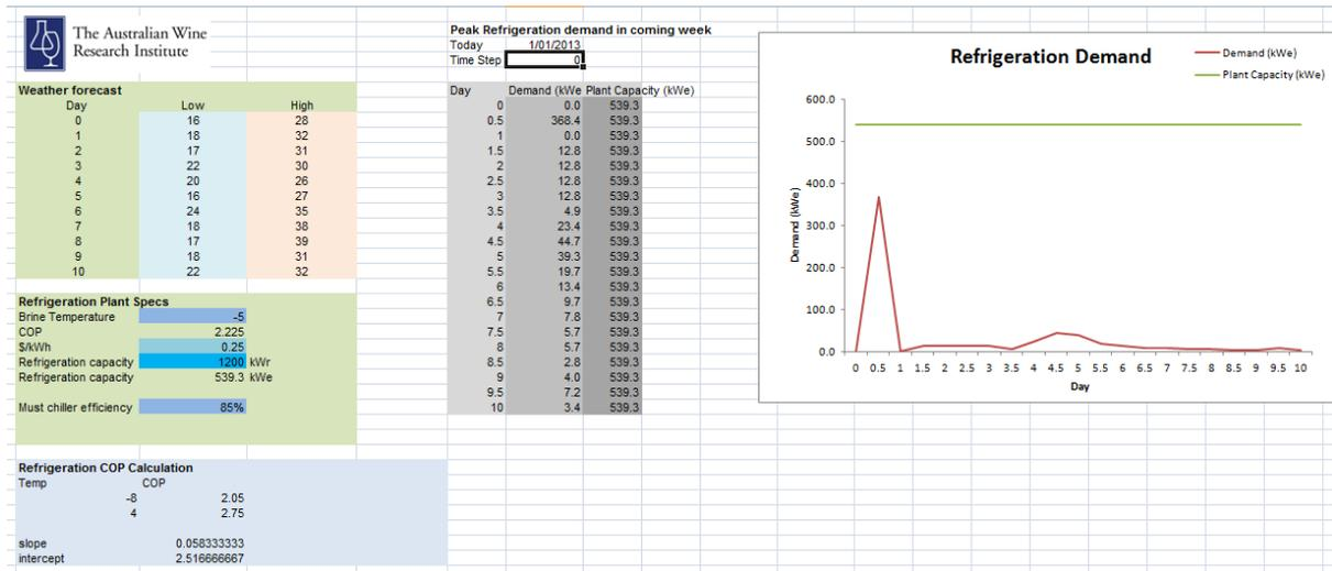
This worksheet gives both a tabular and graphical display of predicted refrigeration demand over the coming 10 days, based on the fermentation data that has been entered into the Simulator. As ferment predictions are made and the results recorded on the Full Vintage Planner, the Refrigeration Demand graph will be updated.
