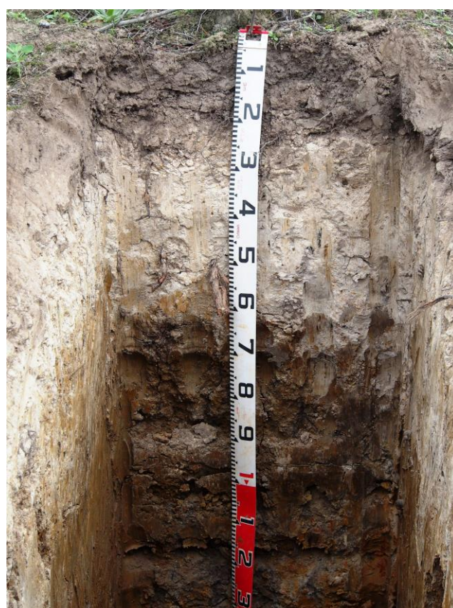
Figure 1 Duplex soil profile showing a sandy loam A horizon over a dense clay B horizon.
