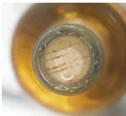
Figure 6. View of the top of the natural cork 'window' bottles. Araldite was applied to the top of the bottle to cover the closure bottle interface. A circle of approximately 30% of the original cork surface area was left exposed in the centre of the closure.
