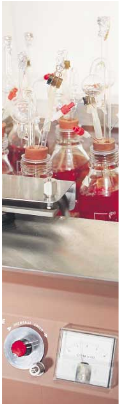
Orbital shaking water bath with small scale fermentations
