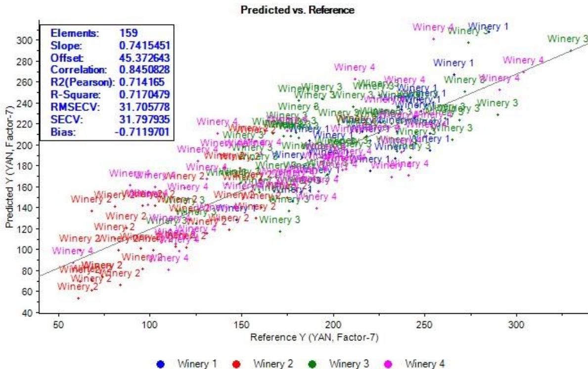
**Figure 5:** Correlation of yeast assimilable nitrogen (YAN) values measured using enzymatic reference method (x-axis) against values predicted using Bruker Alpha Mid-IR spectral method (y-axis). Calibration model includes data from four individual wineries, covering multiple vintages.
