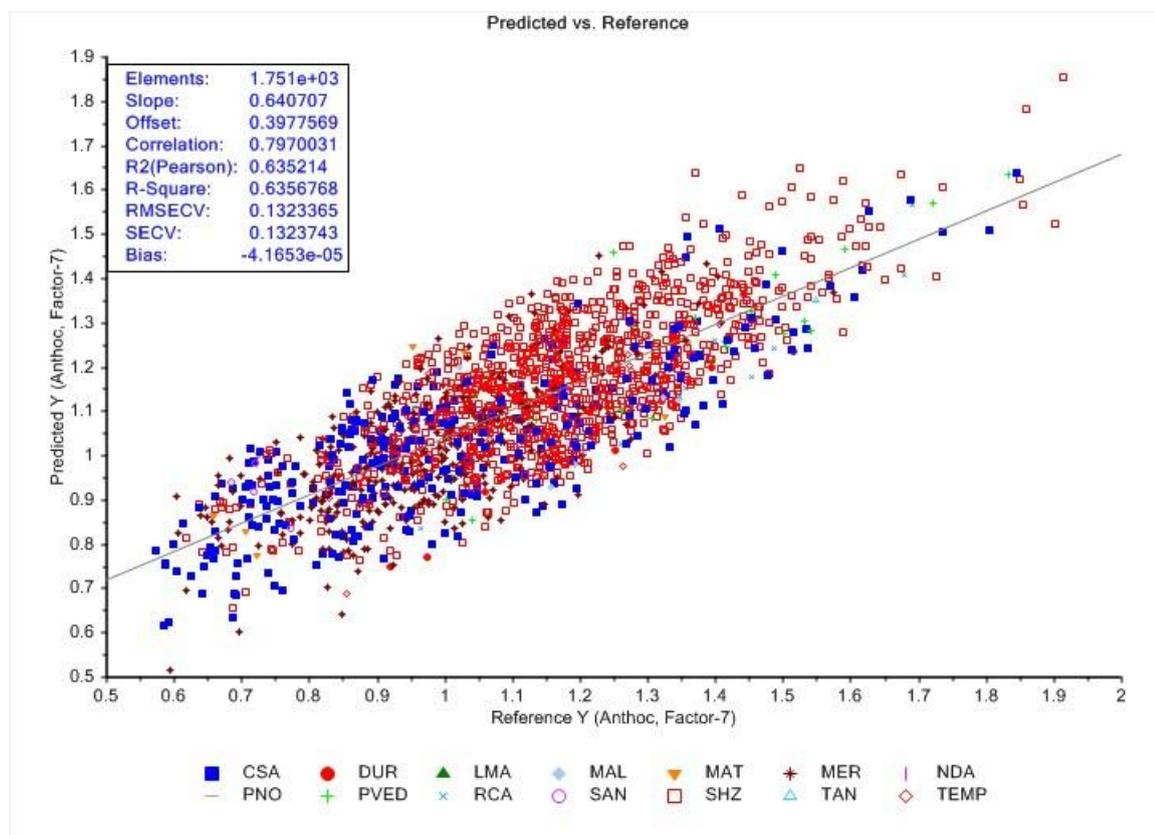
**Figure 3:** Correlation of anthocyanin values measured using Modified Somers reference method (x-axis) against values predicted using Bruker Alpha Mid-IR spectral method (y-axis).
