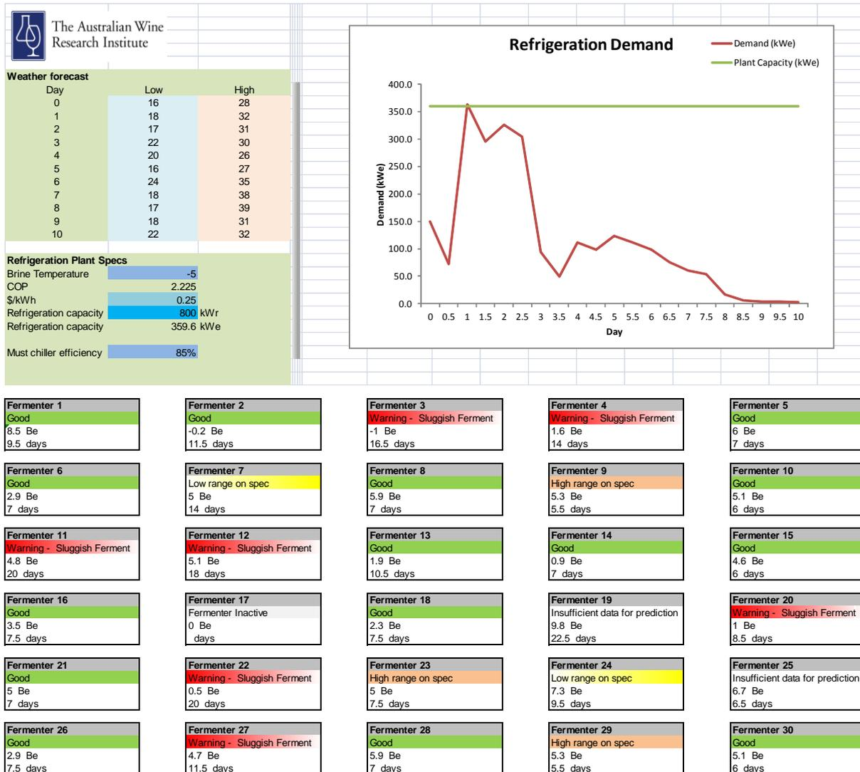
**Figure 4:** An example ferment status screen for a typical commercial tank farm, including upcoming weather forecast and predicted consequential impact on refrigeration demand
