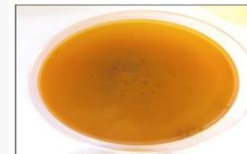
Dispersion score 4: Complete dispersion leaving only sand grains in a cloud of clay
