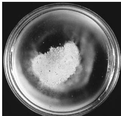
Figure 3: Partial dispersion: the dispersed clay spreads into thin streaks and crescents on the bottom of the container.
