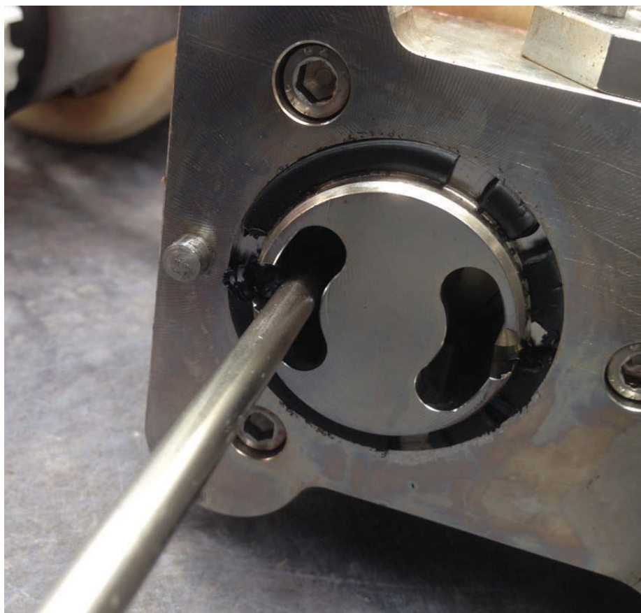
Figure 5. Example of degraded o-ring in filler head component.
