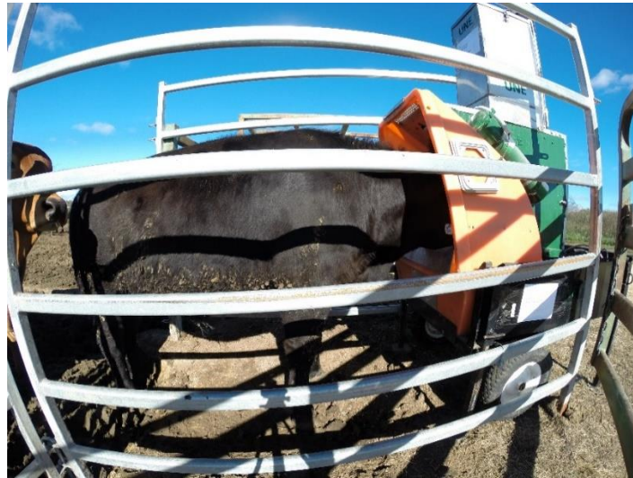
Figure 4: Angus steer accessing the GreenFEED emission monitoring unit for methane measurement.
