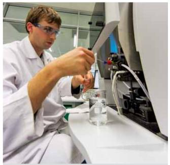
LAB TEST: An Atomic Absorption Spectrometer is used to analyse for manganese at the AWRI. Photo Eric Wilkes.
