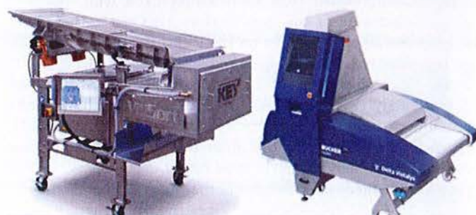
Figure 14: Optical grape sorters (a) Low throughput gravity-fed system with integrated overhead pre-draining screen, (b) High-speed belt conveyor fed system (additional pre-draining screen is required but not shown)
