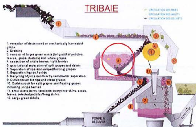
Figure 12: Amos Industrie Tribaie sorting system schematic (density bath circled)
