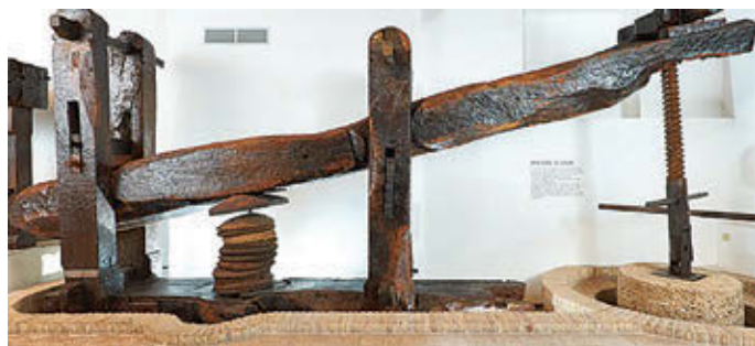
Figure 5. Lever press with screw and counter-weight
