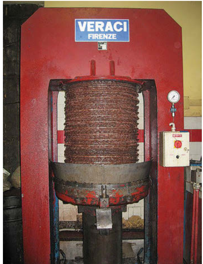
Figure 7. Pressing a stack of olive paste covered mats in a hydraulic press
