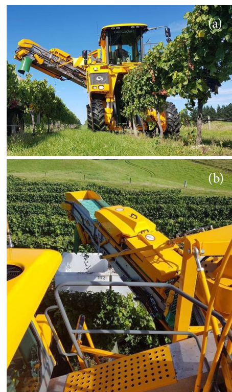
Figure 14. Gregoire EasyClean destemmer mounted on the side-arm discharge conveyor.
