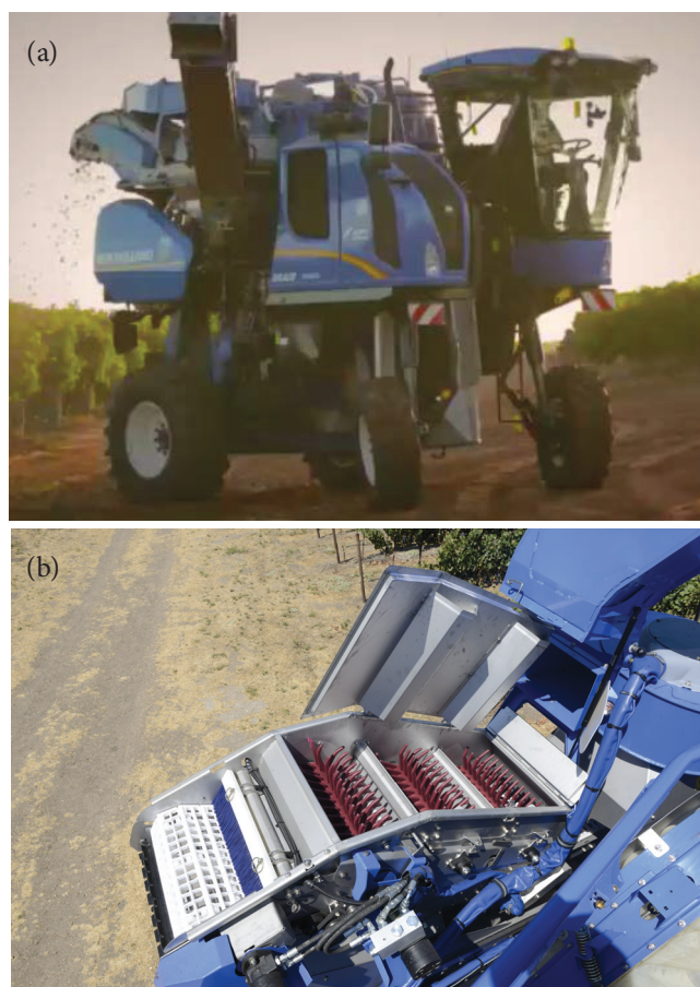
Figure 12. Braud New Holland harvester with SOCMA destemmers and side-arm discharge conveyor: (a) overview, (b) SOCMA finger-wheel destemmer.
