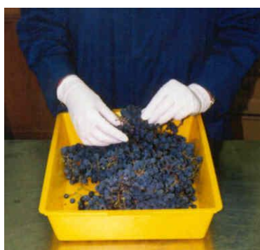
Figure 2. Plucking berries from bunches into a typical 'kitty litter' tray prior to mixing and sub-sampling 500 grams into a zip-lock plastic bag
