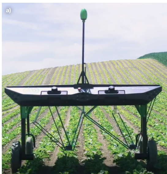
Figure 10. Ecorobotix precision weed spraying robot: (a) 2018 prototype with sprayers on delta arms that move to just above the weed and spray it, and (b) 2019 AVO version with a view of the multi-valve spray-bar underneath the robot that allows for faster operation than with delta arms
