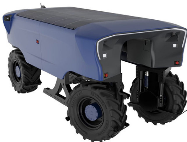
Figure 3. SITIA Trektror – comes in three versions with different adjustable widths: (a) at SITEVI in an over the row configuration, and (b) in a vineyard between rows
