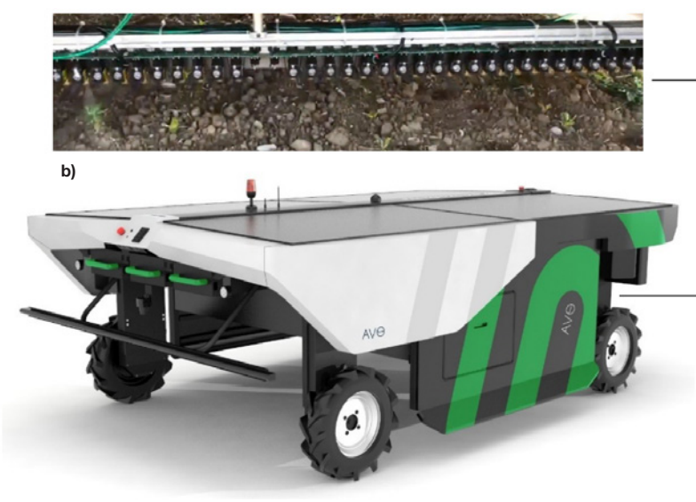
Figure 10. Ecorobotix precision weed spraying robot: (a) 2018 prototype with sprayers on delta arms that move to just above the weed and spray it, and (b) 2019 AVO version with a view of the multi-valve spray-bar underneath the robot that allows for faster operation than with delta arms
