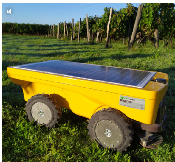
Figure 9. Vitirover mowing robot: (a) In a vineyard, and (b) alongside train tracks
