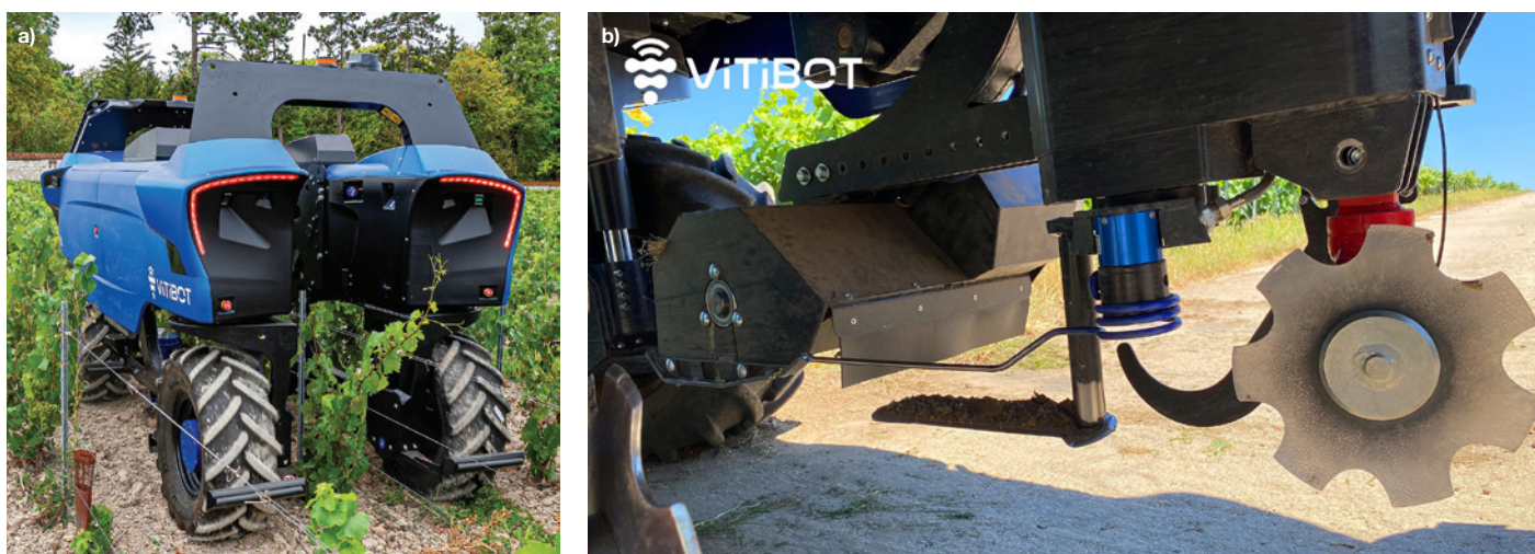
Figure 1. Vitibot Bakus - available in two different sizes to accommodate different vine heights: (a) running in a vineyard, and on a different occasion, (b) underneath view showing one side of the vineyard floor management tools fitted to the robot - a serrated disc, electrically actuated inter-vine cultivator with feeler, and an electric rotary mid-row mower.
