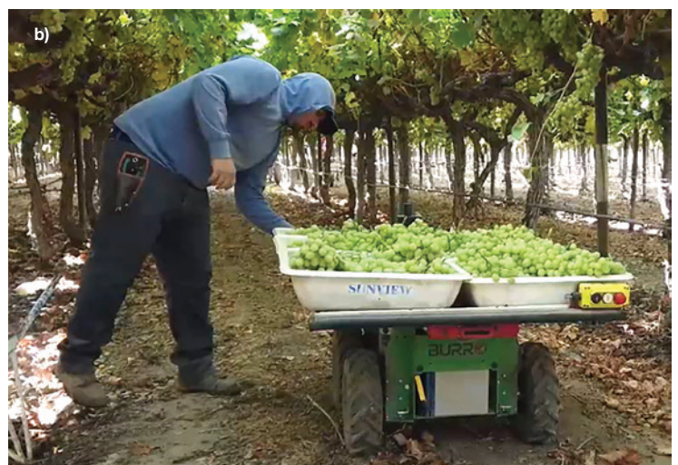
Figure 16. Burro fruit carrying and towing robot: (a) loaded up with blueberries, and (b) table grape picker pressing the screen to send the grapes from the row back to the packing table
