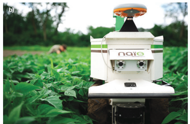
Figure 15. Naïo Oz robot: (a) Old version which relied on red rods to be installed at the end of rows when crops had not yet grown very high so that it knew where to turn for the next row, and (b) new version with guidance by high accuracy satellite positioning (allows passage even without the red stakes or crop growth that other sensors could use to detect where the row is)
