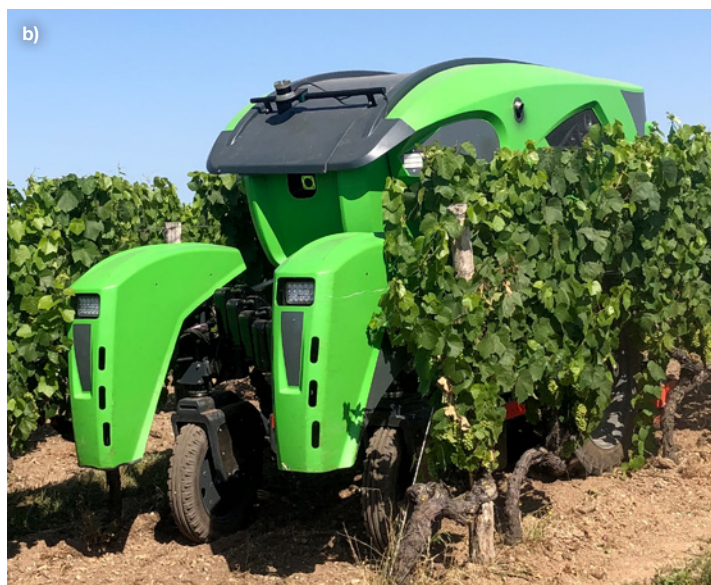
Figure 3. SITIA Trektror – comes in three versions with different adjustable widths: (a) at SITEVI in an over the row configuration, and (b) in a vineyard between rows
