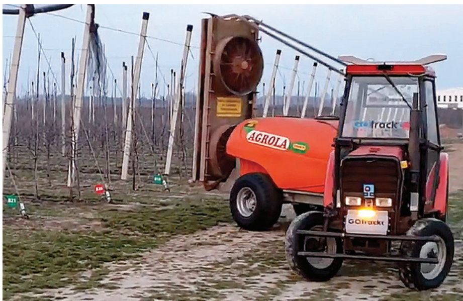
Figure 13. Tractor with GOtrack kit driving autonomously in an orchard (GOtrack 2019)
