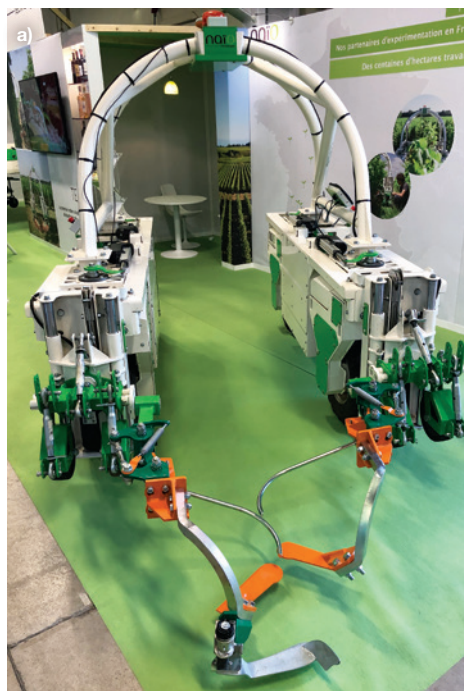
Figure 2. Naïo TED - with under-vine cultivation implements: (a) on display at SITEVI, and (b) in a vineyard
