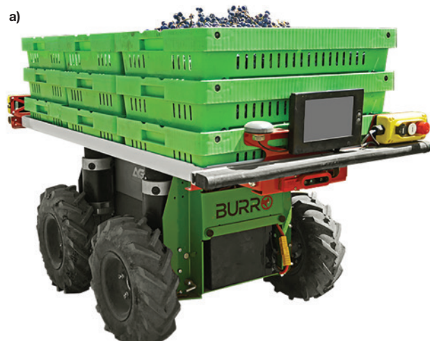
Figure 16. Burro fruit carrying and towing robot: (a) loaded up with blueberries, and (b) table grape picker pressing the screen to send the grapes from the row back to the packing table
