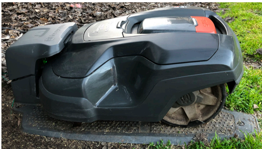
Figure 5. Domestic autonomous lawnmower at its charging station (if the battery is getting low, the lawnmower returns to charge automatically and then goes back to work when the battery is charged)
