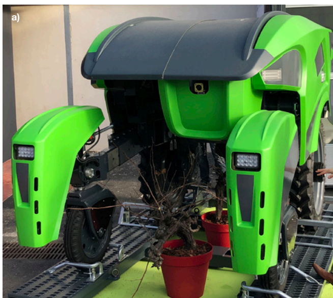
Figure 3. SITIA Trektror – comes in three versions with different adjustable widths: (a) at SITEVI in an over the row configuration, and (b) in a vineyard between rows
