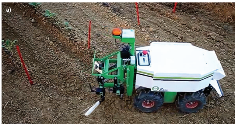
Figure 15. Naïo Oz robot: (a) Old version which relied on red rods to be installed at the end of rows when crops had not yet grown very high so that it knew where to turn for the next row, and (b) new version with guidance by high accuracy satellite positioning (allows passage even without the red stakes or crop growth that other sensors could use to detect where the row is)
