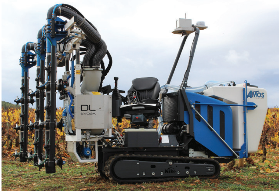
Figure 14. Amos Niko crawler tractor for narrow row vineyards, where remote operation or autonomy has safety benefits when spraying chemicals since the cab is open
