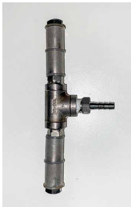
Figure 1. Drop-in t-piece sparger fitted with four 2µm sinters, used for the macro-oxygenation treatments.
