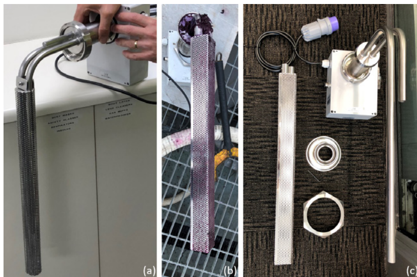
Figure 11. Integrated screens on the Winegrid WP1100 sensor that are able to be installed and removed via the tank fitting: (a) design that fits through a 50 mm DIN fitting, (b) design that fits through a 4-inch BSM fitting and (c) this same design disassembled
