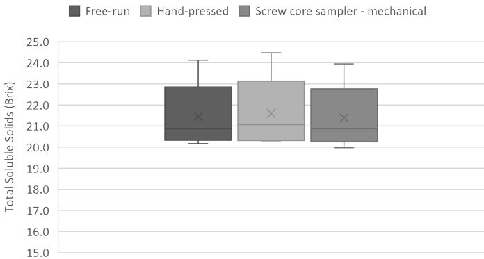
Figure 1. Range of results for total soluble solids (TSS) measured after different sampling/extraction methods for white grapes at Site A. The boxes represent the spread from the first quartile to the third quartile of the data, with the horizontal line within the box representing the median value and the crosses representing the average value. The ‘whisker’ lines above and/or below each box extend as far as the minimum and maximum values measured, excluding outliers, which are represented as dots.
