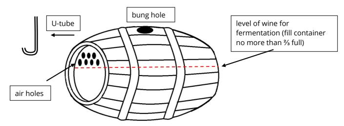
**Figure 1.** Wine barrel with air holes drilled into the heads. All movement of wines into a barrel should be via pumping through a U-tube placed below the surface of the wine. This is to prevent disturbance of the mother culture that forms on the surface of the wine.
