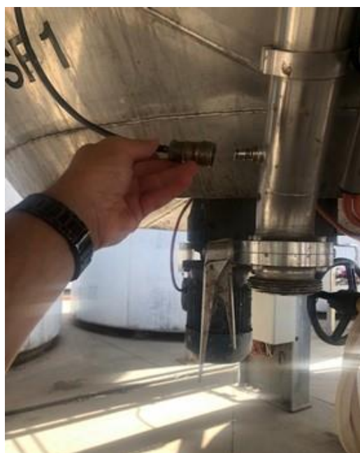
Figure 1. The set-up used for air addition at Calabria Wines, with filtered compressed air delivered via 'nipples' on fermenter rack arms
